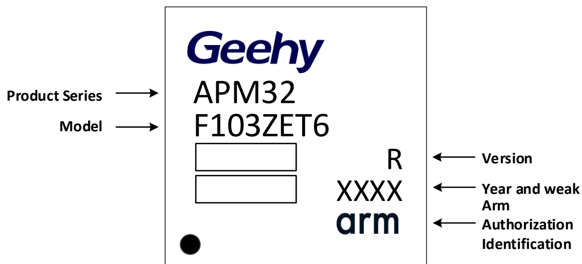
Figure 19 LQFP144-144 pin, 20 x20 mm package identification diagram
