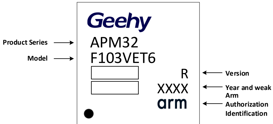
Figure 22 LQFP100 - 100 pin, 14 x 14mm package identification diagram
