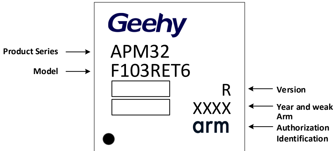
Figure 25 LQFP64 - 64 pin, 10 x 10mm identification diagram
